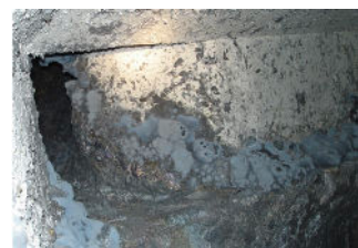
Figure 1 Corundum growth on the refractory lining
