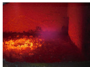
Figure 2 Burner flame impingement creating open area and increased oxidation.
