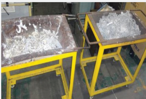
Minimal dross removed after 18 months
